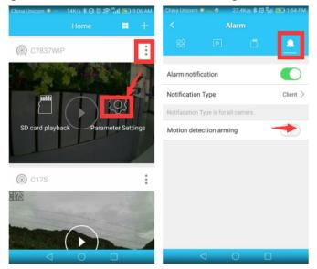
2. Then you can see 'Alarm notification', "Notification Type" and 'Motion Detection arming'. Notification Type. There are two notification type:client and email. Clcik them respectively to view their setup guide, please follow the guide step by step.
