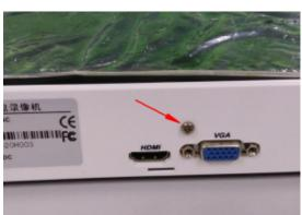
2. Loose and take out all screws, open the top cover, then unistall and remove the battery for more than 5 minitues, reinstall it back,
