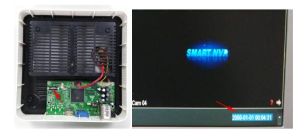
3. 5 minutes later, reinstall the NVR and connect cables, you can see the time (the year 2000) on the display, input the password 000000 to login, then you can modify the password after loginning, please remember these password.
