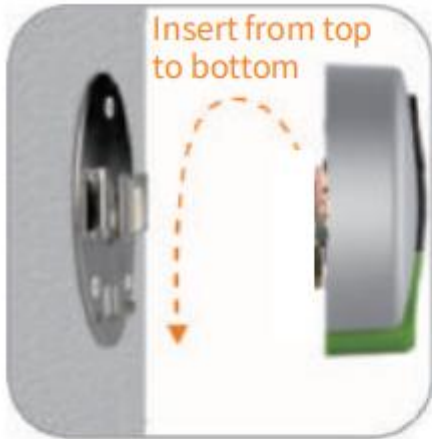
3. Hanging the doorcam on the metal plate
