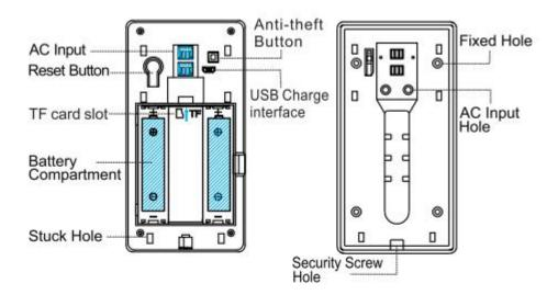
AC Input Power is supplied to the euipment by installing the AC
