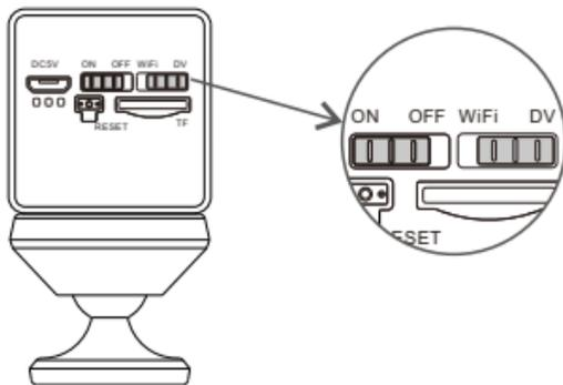
Turn the power switch to "ON", the mode switch button to "DV", and insert a TF card for 24 hours of continuous recording.
