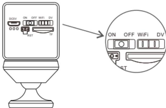
Long press the power switch to turn on the camera, and turn the mode switch button to “DV”, and insert a TF card for 24 hours of continuous recording.
